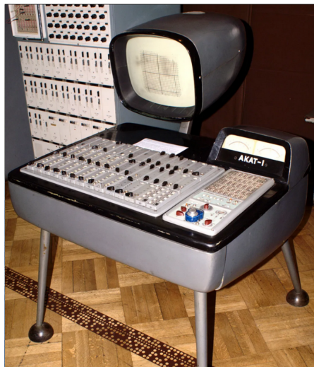
Fig. 1. An Analog Computer: Polish analog computer AKAT-1, from 1959
